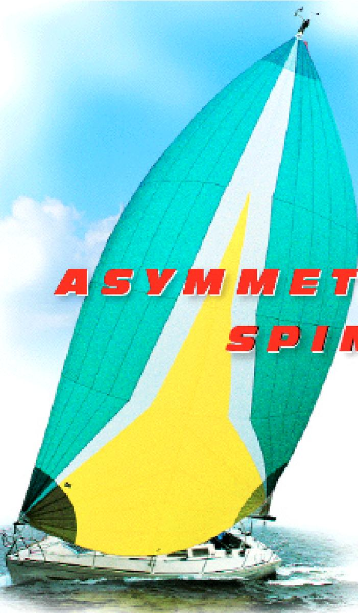
Asymmetrical Spinnakers are a special class of sail that fills in the performance gap between genoas and spinnakers on a boat equipped for a standard spinnaker. On a "Sport" or "Sprit" boat, they are the primary reaching and downwind sails.
