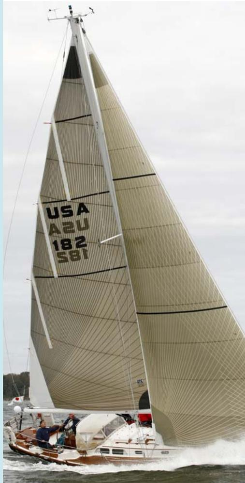
ABOVE: UK-Halsey's VB MaxRoach roller/furling mainsail. TOP RIGHT: The classic 80' yawl MARIELLA with a cross cut Dacron main and standard length battens for her main and mizzen. RIGHT: Reef tack detail on a dacron main.
